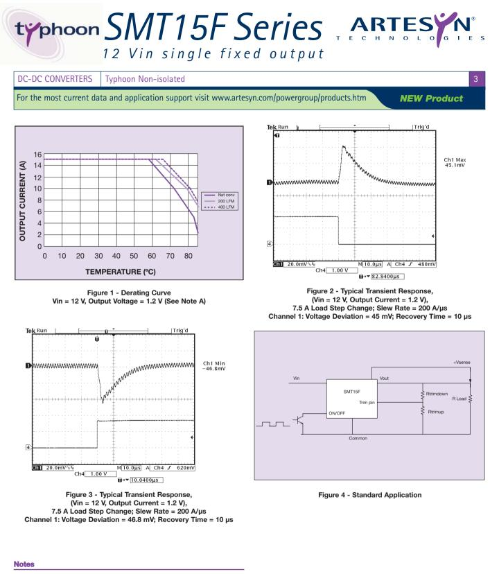
A The derating curve represents the conditions at which internal components are within the Artesyn derating guidelines.
